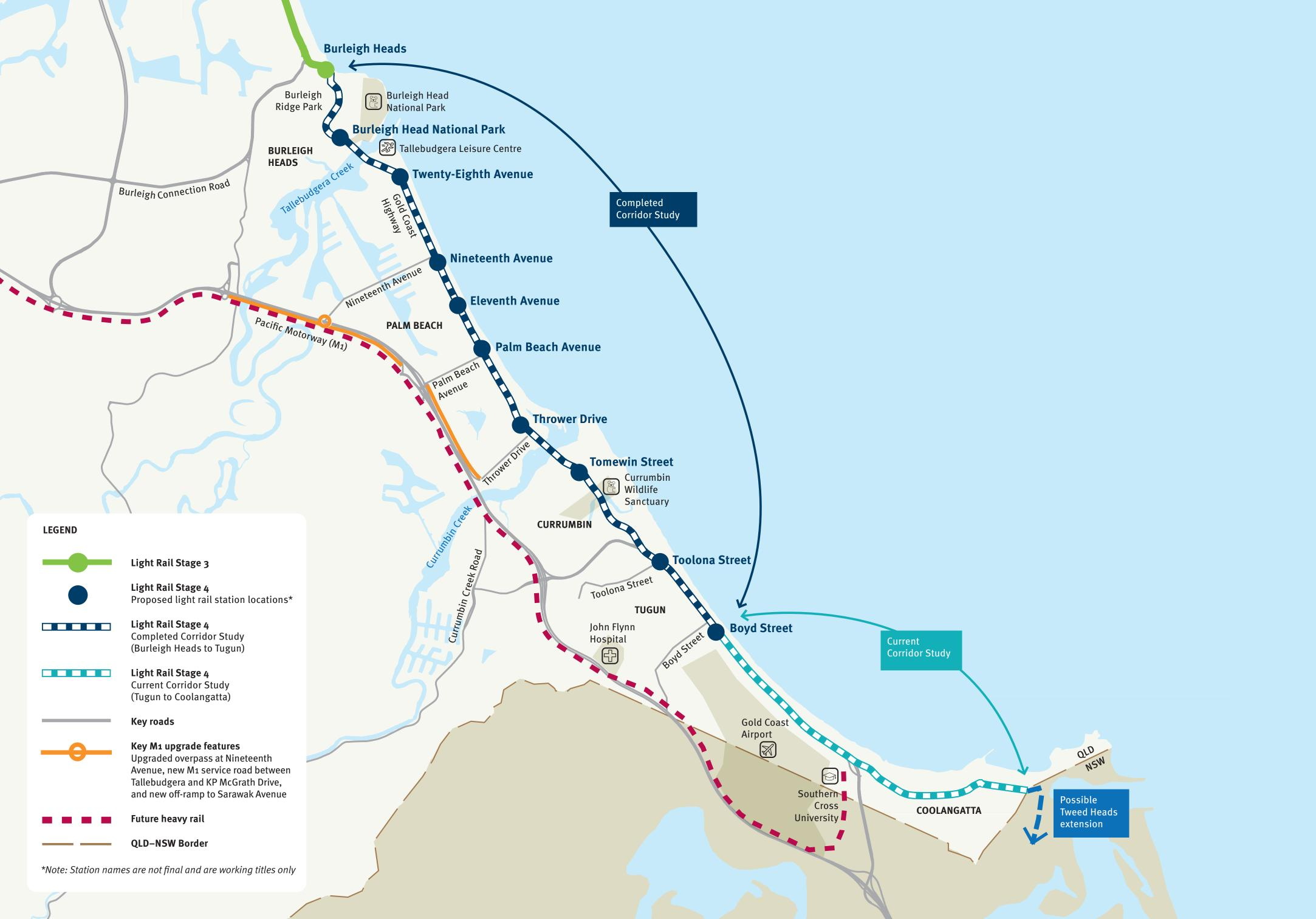
Stage 4 of the Gold Coast Light Rail is a 13 kilometre extension south of the Light Rail Stage 3, linking Burleigh Heads to Coolangatta via the Gold Coast Airport. The Gold Coast Light Rail system is being designed to be delivered in stages to respond to population growth.
